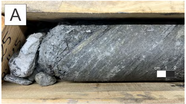
Figure 5. Photoplate showing selected drill core. A: EC024; Semi-massive sulphide with chalcopyrite bands.
