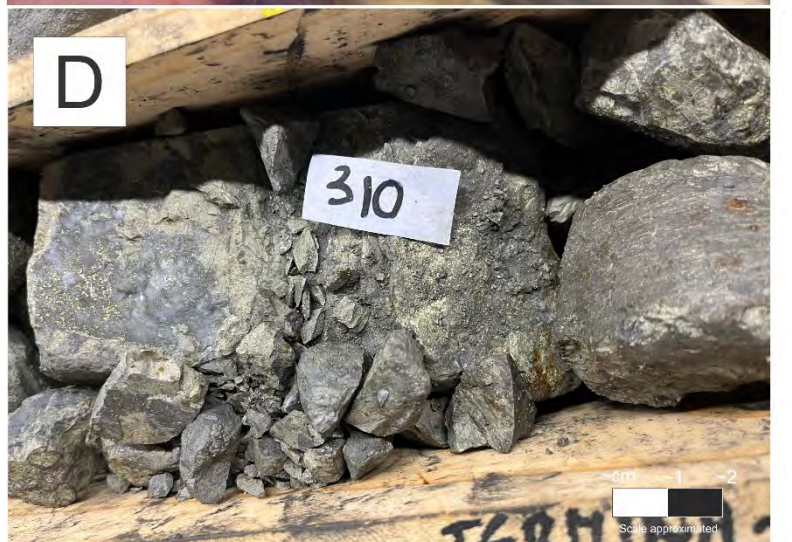
D: EC037; Massive sulphide breccia at 310m in copper-gold rich zone where gold values assayed up to 2.0 g/t Au (see Table 1)
