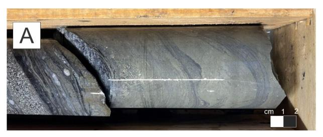
Figure 5. Photoplate showing selected drill core. A: EC039; Massive sulphide with galena, sphalerite and chalcopyrite veins.
