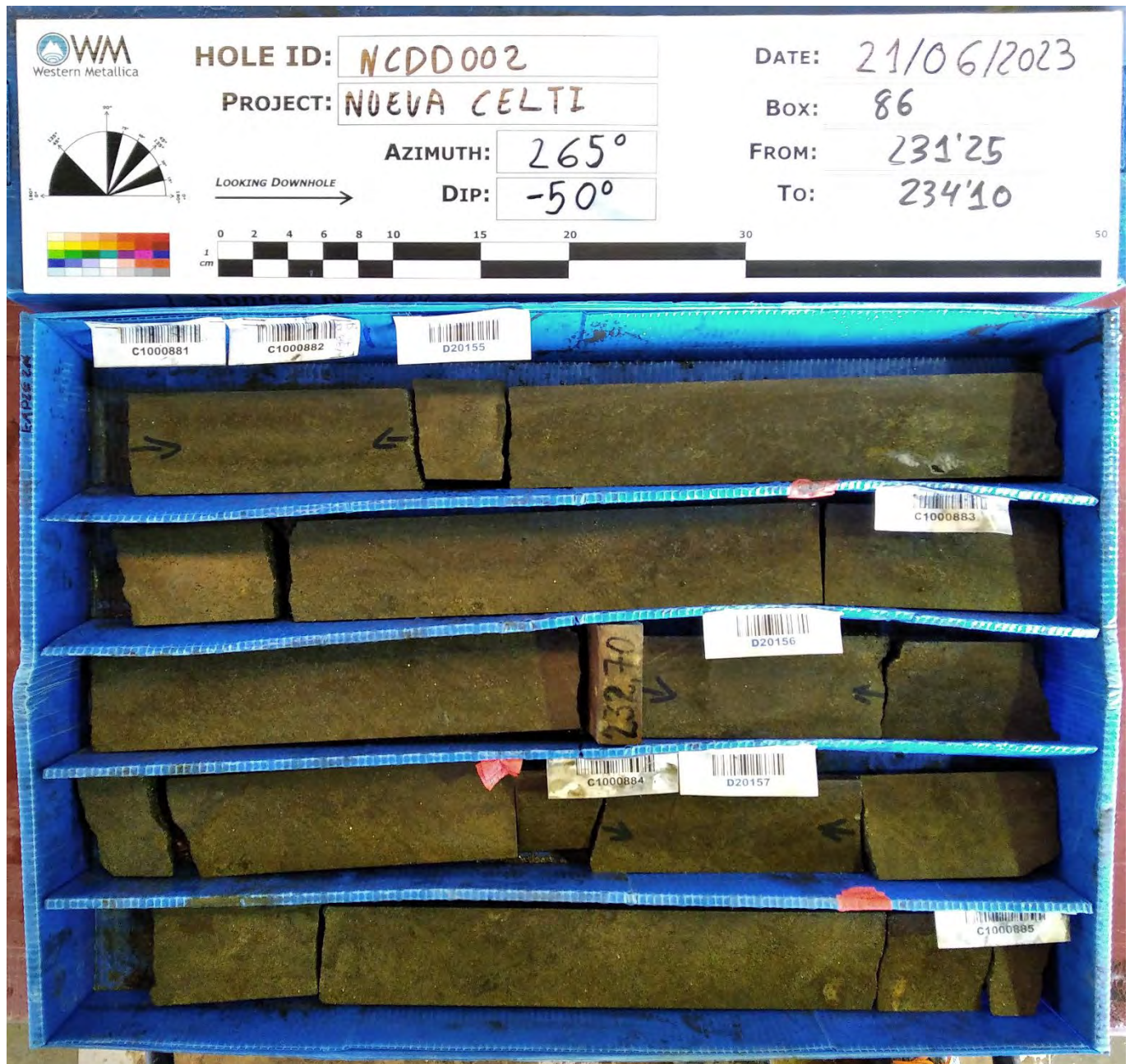
Figure 4. Copper-rich mineralized drill intercept, Nuevo Celti deposit. Deposit remains open at modest depth.
