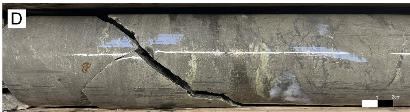
Figure 5 continued. D: EC094 pyritic massive sulphide with abundant chalcopyrite as veins and crystals associated with quartz veining.
